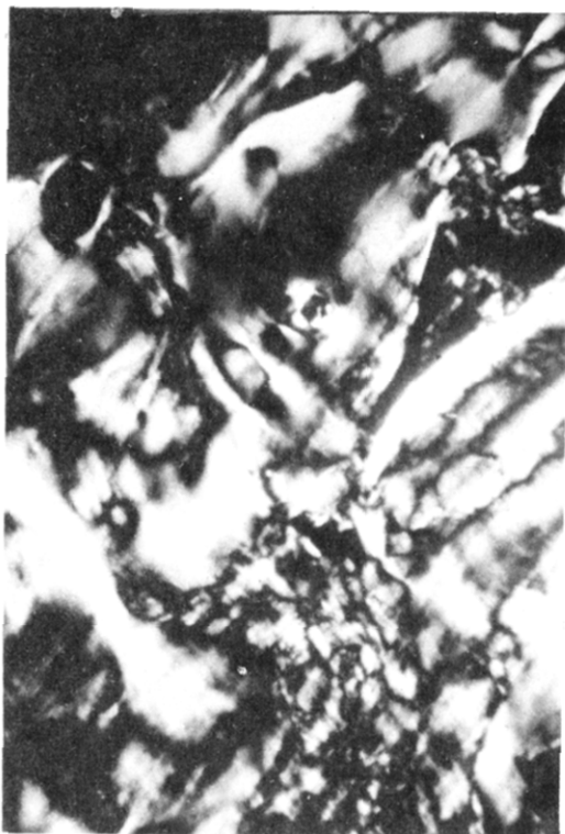
Figure 10. Photomicrograph of 15% (wt) cellulose in 9% LiCl/DMAc showing a large birefringent region under cross-polarizers at 320 \times (reduced to 60% of the original).
